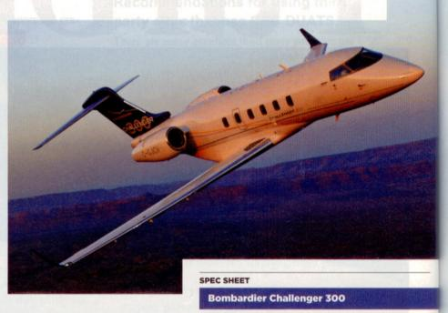
Engines | Two Honeywell HTF7000 turbofans, 6,826 lbs thrust each Seats | 8-9 passengers Max takeoff weight | 38,850 lbs Long-range cruise speed: 458 kt Takeoff distance | 4,810 ft Landing distance | 2,600 ft Range (with IFR reserves) | 3,065 nm Wingspan | 63 ft 10 in Length | 68 ft 7 in Height | 20 ft 4 in
